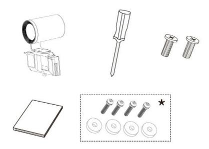
\*Only 12X, If the camera interferes with the wall, please refer to MeetingBoard Wall-Mounted to install the gasket on the back of the endpoint.
